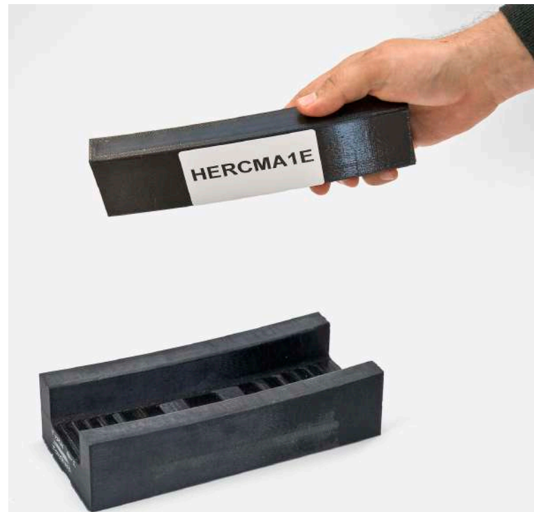
3D printed forming tool in Stratasys Nylon 12.
