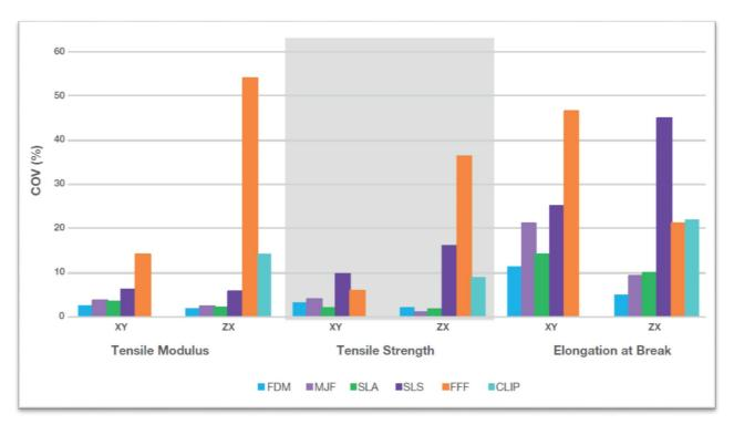
The chart above shows that FDM has the lowest COV in overall mechanical properties. MJF and SLA were good in Tensile Modulus and Strength but not in elongation variance. This means that a manufacturer could design a part for FDM and trust that the mechanical properties won't vary from part to part.
