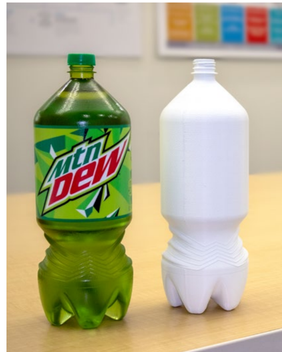
Full color 3D printed prototype next to an all-white printed prototype
