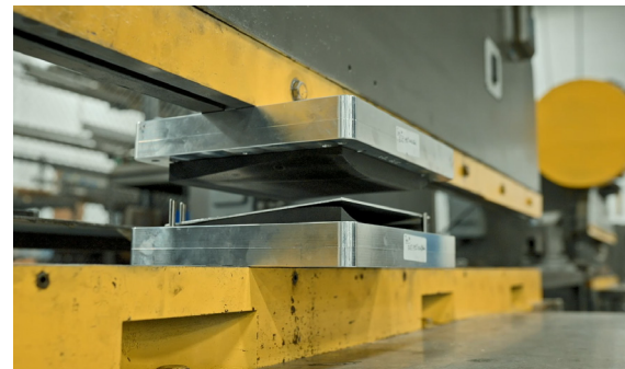
A sheet metal part is about to be formed with the 3D printed dies.
