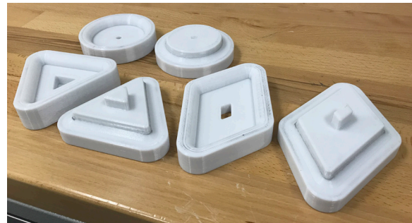
Figure 2-4: Custom flare tooling printed using polycarbonate.
