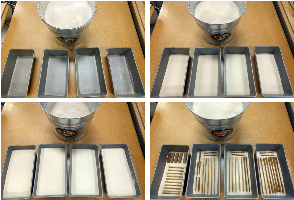
Figure 2: Samples should be placed in a sand bath to prevent deformation while being annealed.
