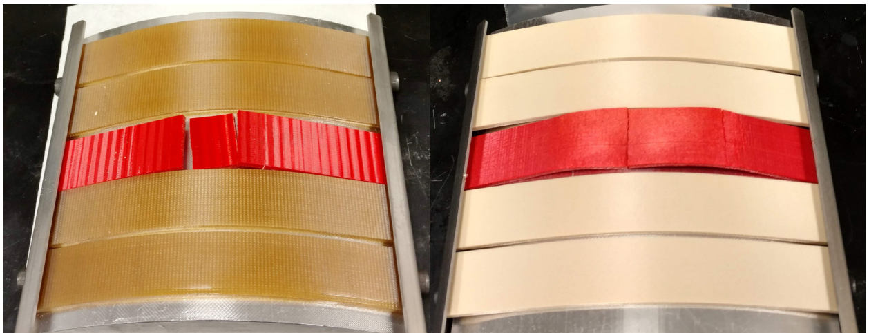
Figure 11: Non-annealed (left) and annealed (right) specimens after exposure to Toluene (orange = ULTEM 9085 resin)
