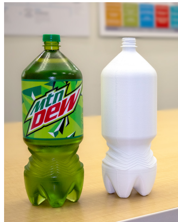
Full color 3D printed prototype next to a low-fidelity 3D printed prototype
